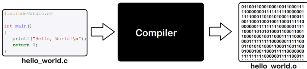
Figure 1: Compilation Process of a C Program
